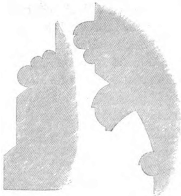
Cap and Base of Pillar, south side of Nave.
