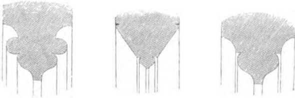
Mullions of Windows in South Aisle
