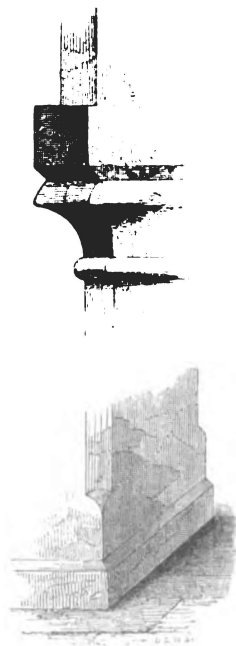
Cap and Base of Pillar in Nave.
